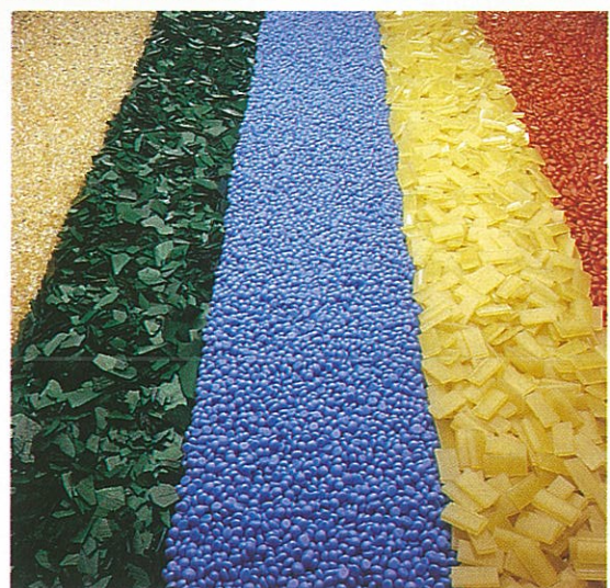
In Sandvik's belt cooling systems, molten materials such as sulphur, waxes and resins are transformed into pastilles, flakes, strips etc.
