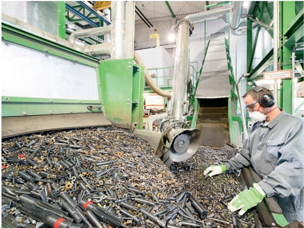
Recycling of cemented-carbide tools at the Wolfram Bergbau und Hütten site in St. Martin, Austria.
