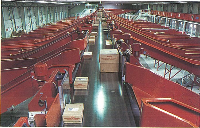
World-wide, more than 15 million packages are distributed on Sandvik steel-belt sorting systems.
