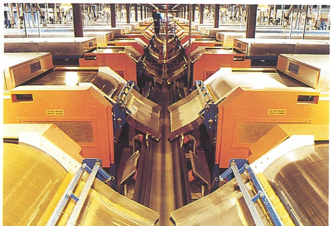
The world's largest facility for converting sulphur into easily handled pastilles, at Shell Canada, contains 46 Rotoform units.
