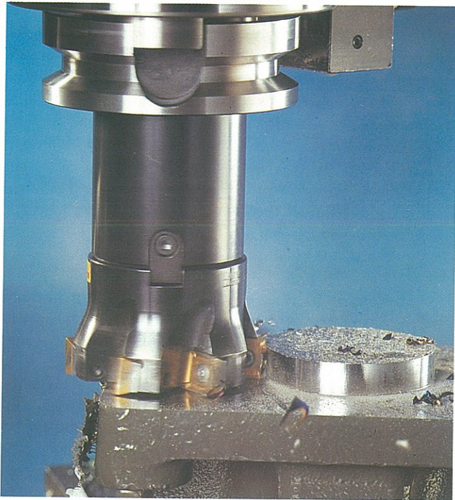
Sandvik Coromant's new milling cutter T-Max 290 offers features that are ideal for machine shops producing short series and, accordingly, need to reduce set-up times.
