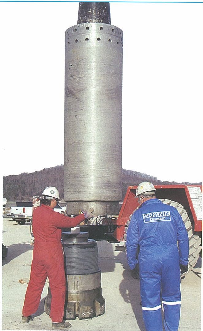
The Hammerdril XL 24, one of the largest and most powerful down-the-hole hammers in the world, can drill holes more than one meter in diameter.
